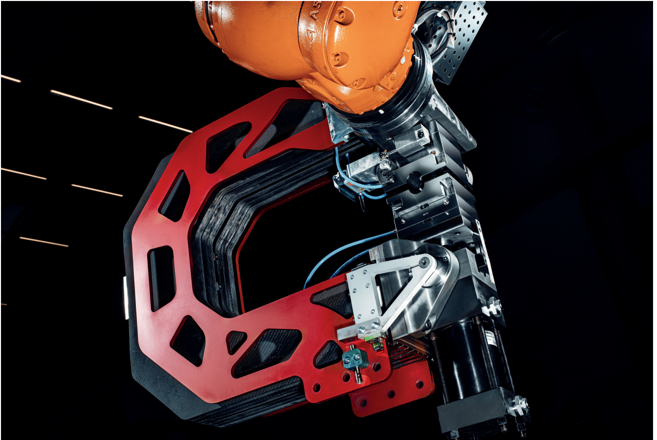
The Robin injection molding system can be swiveled freely on the arm of a six-axis robot to the particular application points. © Anybrid
